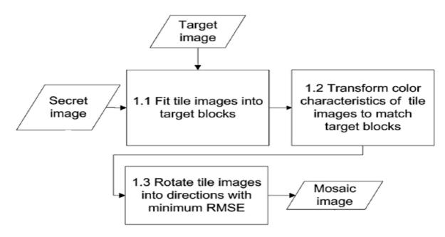
Fig 1: Flow diagram of the proposed method.
